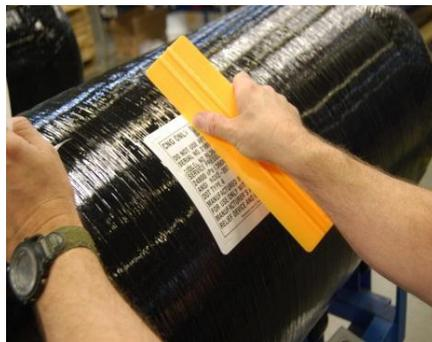
**Figure 3.** Work the label so it conforms to the composite ridges.
