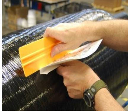
**Figure 2.** Press downward with the plastic squeegee while removing the backing.
