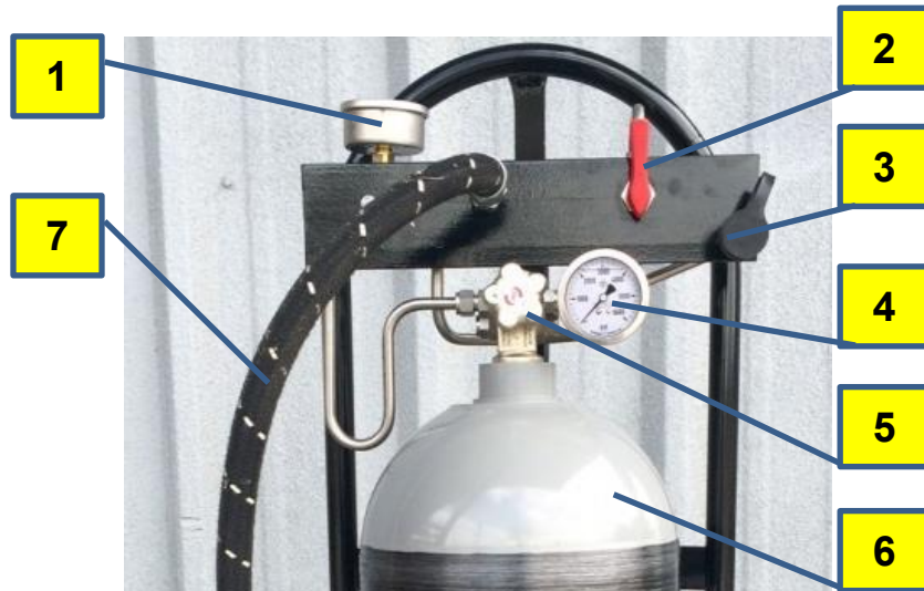
Figure 1. Major components, front view: (1) low pressure gauge, (2) ball valve, (3) fill receptacle and dust cap, (4) high pressure gauge, (5) manual valve, (6) CNG cylinder, (7) flex hose, 20-ft.
