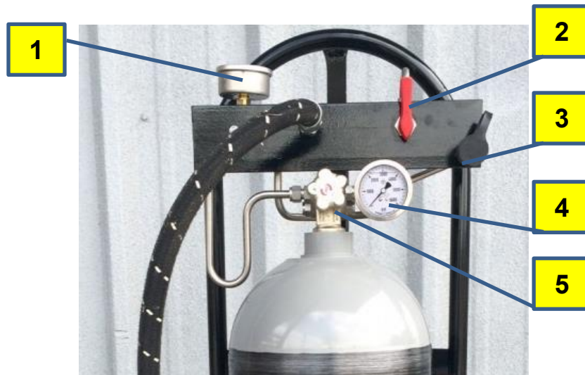
Figure 3. Pony Tank controls: (1) Low pressure gauge, (2) 2-way ball valve, (3) re-fuel receptacle, (4) high pressure gauge and (5) manual cylinder valve. Not shown: Regulator handle, located at the rear.
