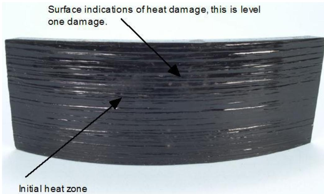
**Figure 4.** The same composite sample in Figure 3 but has been cleaned. Notice the areas of damage visible in Figure 3 are more difficult to identify.
