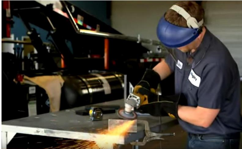
*Figure 1. Welding, grinding and other “hot work” can be safely performed on or near a natural gas vehicle – but certain precautions must be followed.*
