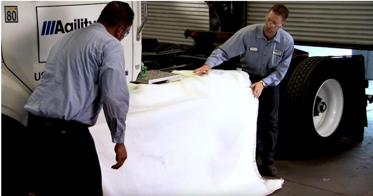
**Figure 2. Cover all CNG or LNG fuel system components with fireproof welding blankets or a metal shield before performing any hot work operation.**
