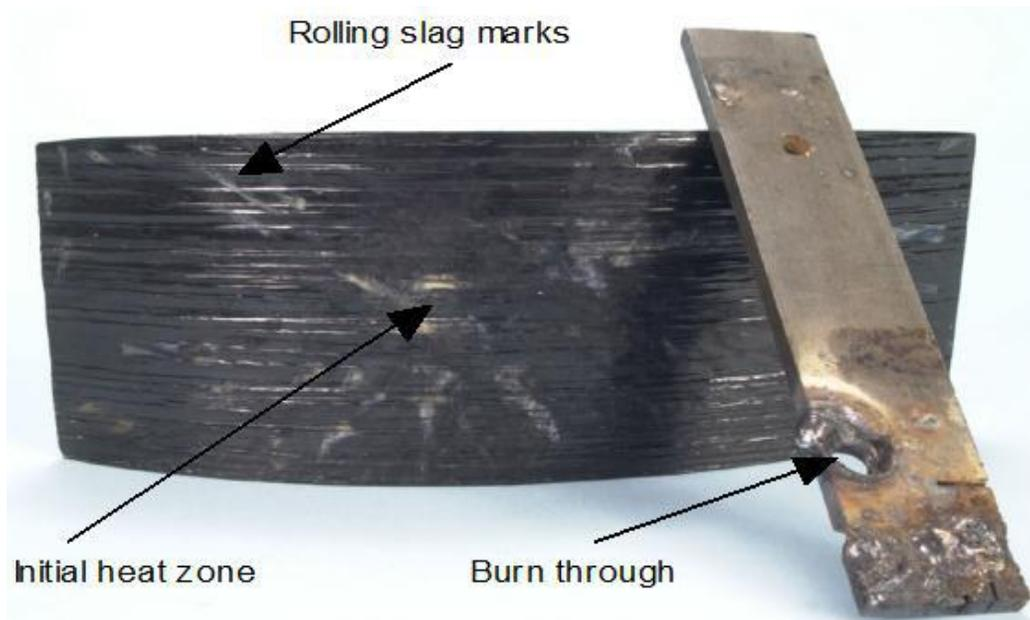
**Figure 3. Composite sample that was subjected to hot weld slag. A 1/4-in. x 1-1/2-in. bar stock was burned through with a cutting torch at a height of 6-in. above the composite sample.**
