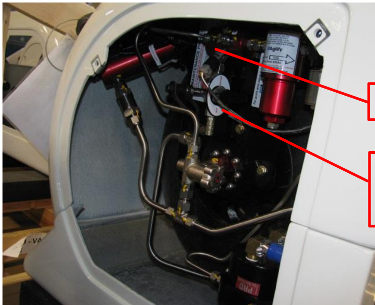
Figure 4 Side mount system connections for fuel transfer. Your configuration may differ from this example.
