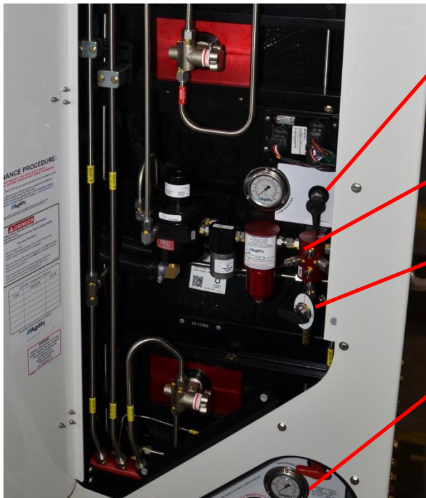
Figure 5 Back of cab system connections for fuel transfer. The bleed valve is mounted on the manifold. Your configuration may differ from this example.
