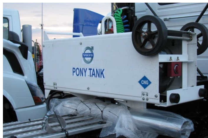
Figure 7 Pony Tank 24400000 can be temporarily mounted on the vehicle to supply fuel to the engine while the vehicle is under construction. Note, Pony Tanks are not approved for use on public roads.
