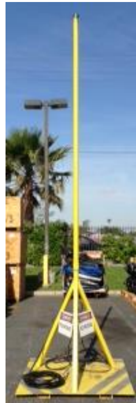
Figure 1 Left: Agility Fuel Solutions Pony Tanks are used as a temporary fuel supply; at right is an example of a vent post for defueling.
