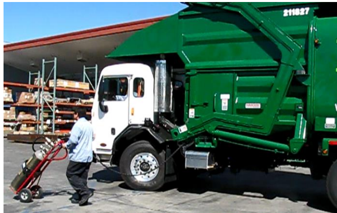
Figure 6 Pony Tank 24403000 being used to move a completed refuse vehicle out of the shop and to a staging area.
