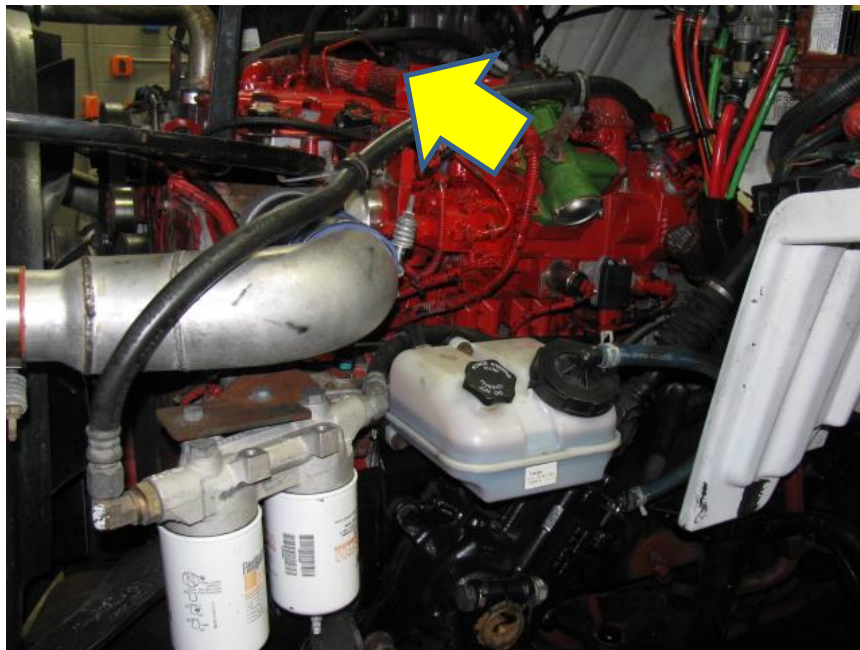
Figure 5 Connect the hose from the Pony Tank to the low pressure filter inlet at the engine.
