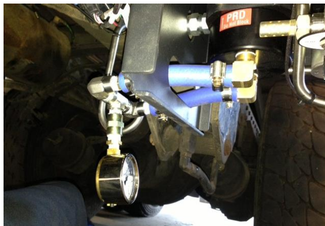
Figure 3. Pressure regulator test setup.
