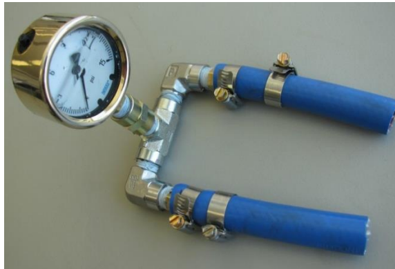
Figure 2. Pressure regulator test jig.
